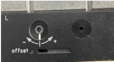
Detailed view of offset adjustment screw.
