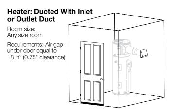
Heater: Ducted With Inlet and Outlet Duct
